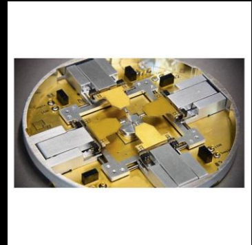
Manipulator Robot we used to get measurements of our sample chip in the SEM.
